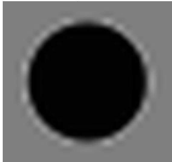
(b) Zoomed view of the largest hot sphere (sphere 6). Ringing artifacts are apparent outside the wall of the sphere, and the top and bottom of the sphere wall appear to be truncated. A complex ringing perpendicular to the sphere wall has been observed on some displays.
